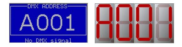
It shows the emulation of the display panel mounted on the fixture selected; by using the four buttons (chapter 5.6) the emulation of the display will show all the pages of the menu as facing the real display.
