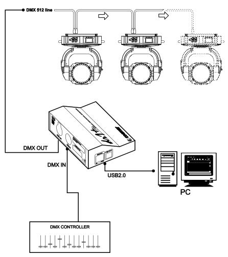
It is possible to connect all **Coemar** devices, only if each device has its own ID number and is equipped with DMX and/or Artnet connector.
