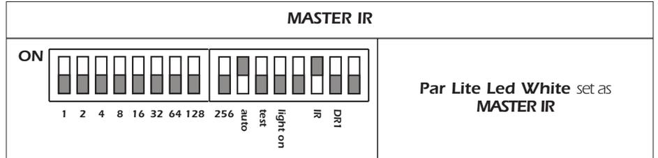
To configure a **Par Lite Led White** as **MASTER** set the **IR and Auto** dip-switches to **ON**.
