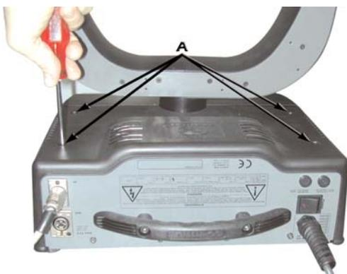
1. Loosen the screws on the cover of the base of the unit, as shown in the diagram below, using an appropriate screwdriver, thereby removing the cover completely and allowing access to the internal components of the base of the **iWash Halo**.
