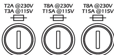
4. If the voltage setting is 115V replace the fuses located on the rear panel of the base. The fuse T2A, suitable for 208/230/240 V, must be replaced with a fuse T3A, and the two fuses must be replaced by two fuses T15A. The fuses are in a plastic envelope together with this instruction manual.
