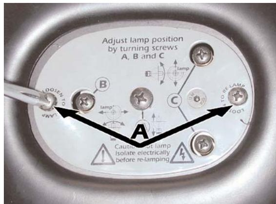
2. Remove the lampholder assembly "B".
