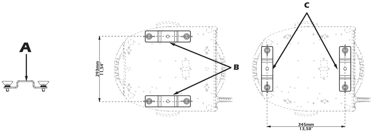
For ceiling mounted installations we suggest the use of appropriate clamps or fixings to attach the fixture to the mounting surface. Clamps may be attached to the central hole provided in the cam-lock brackets, as shown in the following diagram.
