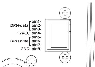
On rear panel of **iWash Halo** base you find a RJ45 connector, as shown in picture, that can be used either for display supply and for software upgrade function.
