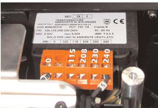
2. Locate the transformer in the base of the unit.
