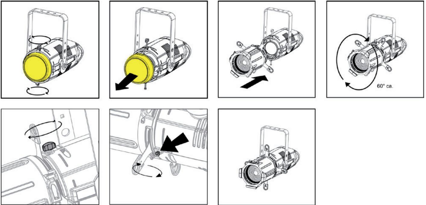
Remove the frontal cap by loosening the upper and lower screws enough to free the cap itself, set the optic's flange tilted about 60°. Insert the optic's flange into the body's receptacle and turn the optic 60° until it is firmly assembled to the projector body, free to rotate but not free to detach itself from the body. Ensure the optic to the body by tightening the two screws previously loosened.
