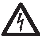
1. Presence of high voltage inside of the fixture. Insulate the projector from mains supply before opening or performing any function which involves touching the inside of the fixture, including lamp replacement.
