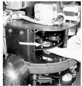
2) Reverse the procedure to install a replacement gobo.
