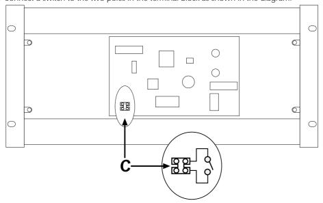
3) Connect a switch to the two poles in the terminal block as shown in the diagram.
