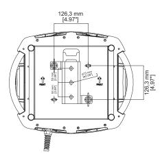
For ceiling mounted installations we suggest the use of appropriate clamps or fixings to attach the fixture to the mounting surface. Clamps may be attached to the central hole provided in the cam-lock brackets, as shown in the following diagram.
