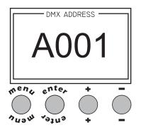
Important Note: holding down the + or - buttons will cause the display to alter at an increased speed, allowing a faster selection to be made.
