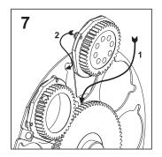
The gobos wheel only accepts gobos with the following features: External diameter 27 mm Working area diameter 21 mm Thickness: metal gobos from 0,2 to 0,5 mm, glass gobos up to 4 mm
