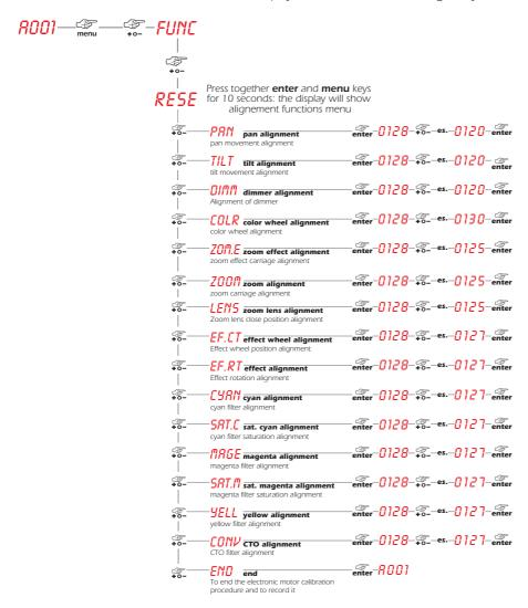
**Note:** Simultaneously pressing the + and - buttons will return the calibration value to 128 (default).
