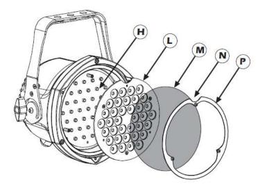
To further increase the beam angle, the "R" reflector is available (cod. CO9168) and it must be fitted instead of the lenses group and filter holder.
