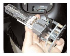
5. Replace the lampholder assembly in its original position and refasten the two screws "A" which were previously removed.
