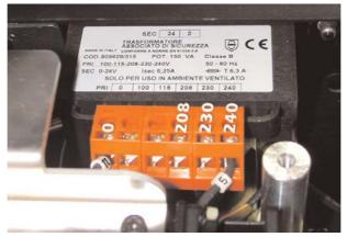
Select a voltage from amongst 208, 230 or 240V by disconnecting cable n° 5 and moving it to the correct voltage. Refer to the sticker located on the transformer to ensure the proper terminal is selected for your requriements.
