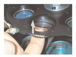
**5.** Repeat the above procedure in reverse to replace a gobo into the gobo wheel.
