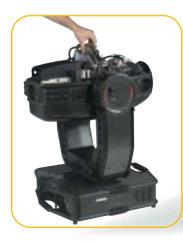
Modular construction allows the lighting designer to personalise fixtures to suit specific applications, even during rehearsals, when access to luminaires may be limited. All of the modular components are easily removed via simple, quick-release 1/4 turn captive wingnuts. Each component is equipped with slot-in electrical and electronic connectors which are vibration-resistant, same as those used in the automobile industry.
