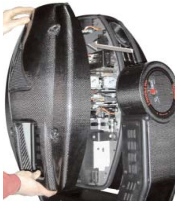
Figure W11B Removing Top Cover
