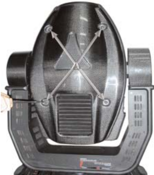
Figure W11A Removing Top Cover
