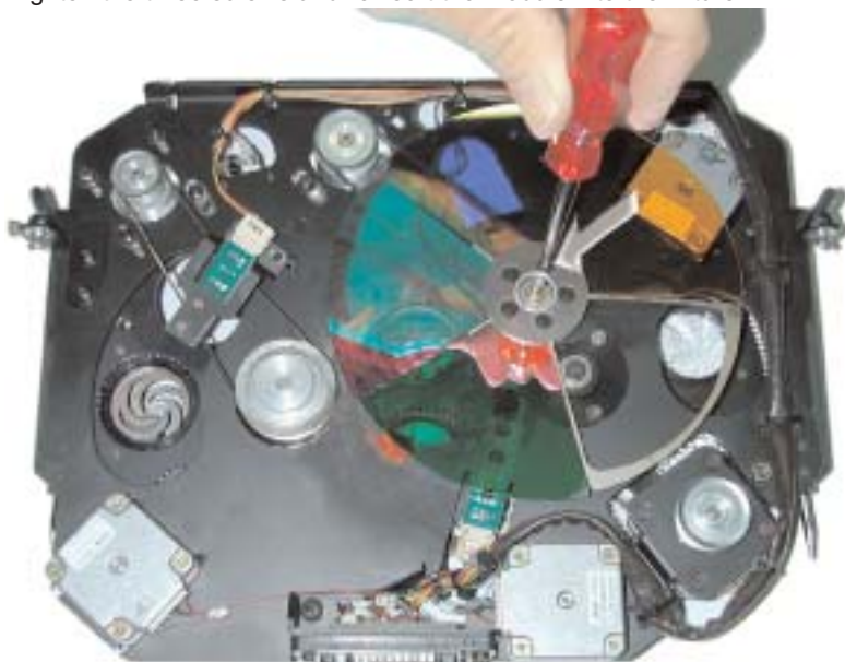
Figure W16B: Loosen Screws on Color Wheel
