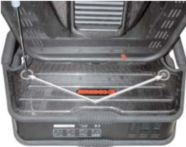
Figure W12A: Removing Base Covers
