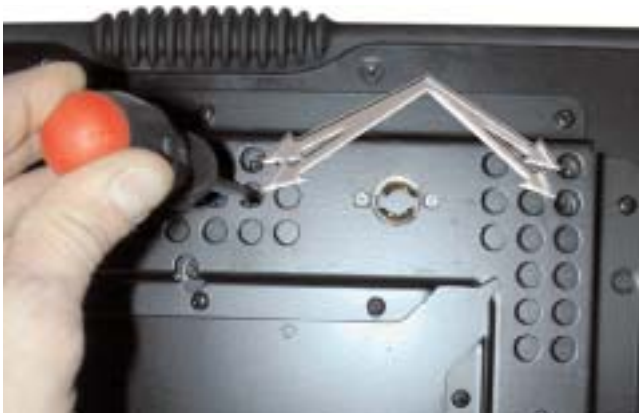
Figure W12C: Removing Switching PS screws
