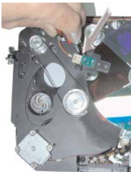
Figure W16A: Removing Sensor
