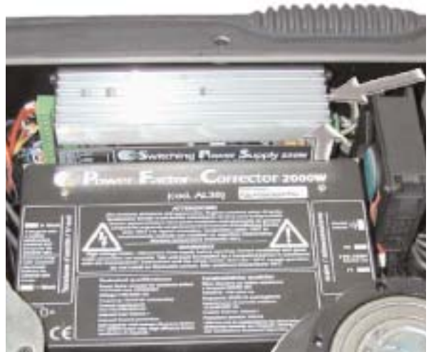
Figure W12B: Locating Switching PS
