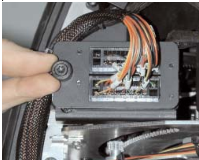
Figure W15: Disconnecting Color+Gobo+Effect Module Harness
