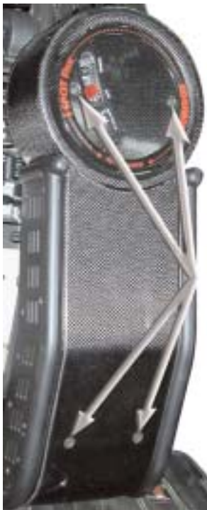
Figure W13A: Removing Arm Covers
