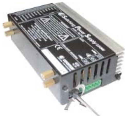
Figure W12D: Removing the Switching PS Fuse
