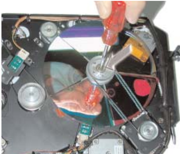
Figure W16C: Loosening Color Wheel Screws
