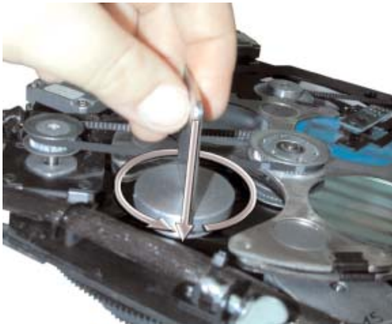
Figure W17 Remove Retaining Ring using Gobo Tool
