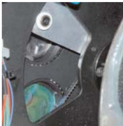
At this point proceed as per section A (**replacing gobos on gobo wheel 1**). Following this, proceed as in section B (**replacing gobos on gobo wheel 2**), following the procedures shown in Fig.5 and in Fig.4, sliding the lever in the opposite direction in order to close up the opening and retightening screw **D** as shown in Fig.4
