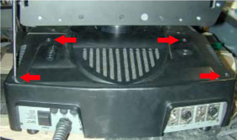
2) Locate the autotransformer in the base of the unit.
