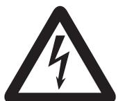
1. Presence of high voltage inside of the fixture. Insulate the fixture from mains supply before opening or performing any function which involves touching the inside of the fixture, including lamp replacement.
