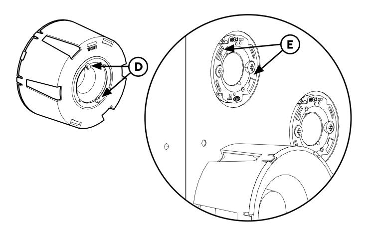
Turn clockwise until the lens is perfectly fitted.
